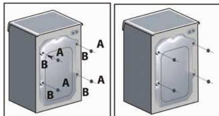
**Note:** we recommend you keep the spacers and screws to immobilize the machine for future transit. The Manufacturers will not be responsible for any possible damage to the machine caused by not following the rules relating to releasing the mechanism. The user is responsible for all costs of installation.
