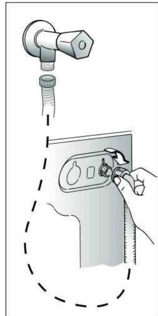
If the inlet hose's connection point is changed, check that the  $\frac{3}{4}$ " threaded ferrule on the inlet hose is firmly attached to the electrovalve connector.
